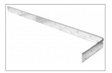
H and L straps are designed to The Building Regulations, BS 5268 Part 3 and other building standards for vertical and horizontal restraint when connecting timber floor and roof systems to masonry walls.
